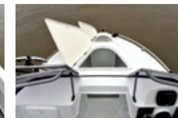
Access to the anchor hatch is via the open window.
